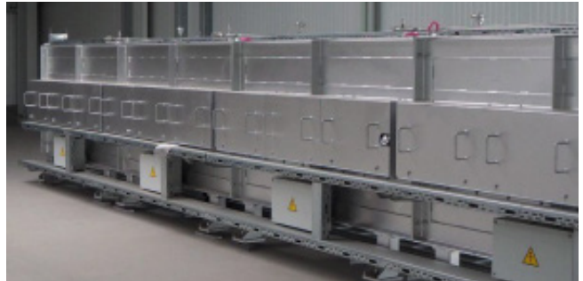
Heating section for heating air from 300 °C to 1,100 °C.
