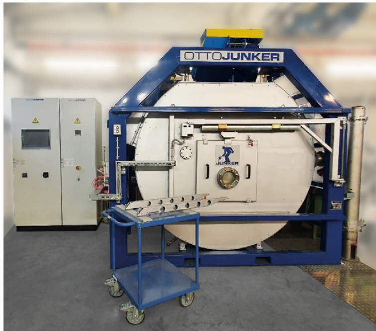
Pilot plant for the thermal recycling of batteries
